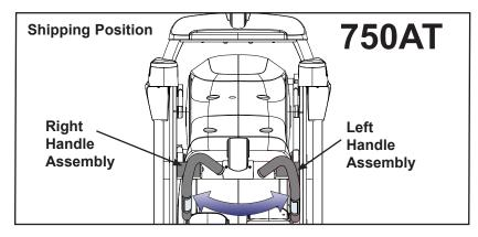
1. Locate the screws and washers that secure each handle assembly to the main frame.
