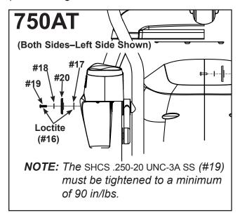
8. Verify handle assemblies are now installed in the correct position.
