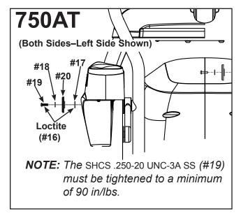
3. Place right handle assembly in position and slide pivot pin back in place.
