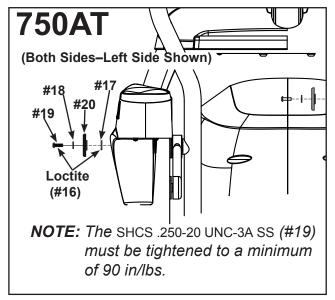
2. Apply loctite (#16) to threads inside the arm and screws removed in step two of **Remove left and right handles**.
