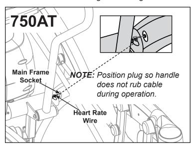
2. Plug right heart rate cable into main frame socket. Refer to the above diagram.
